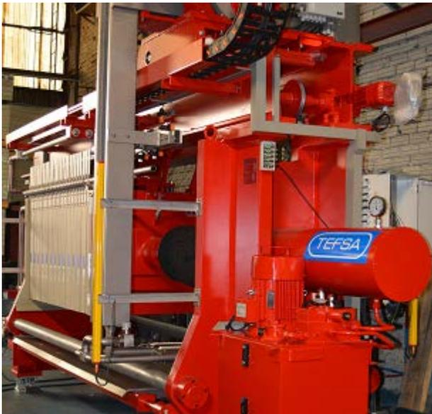
Obviously, the parts in contact with the product can be lined with several protective materials in order to avoid any product contamination or any corrosion on the filter frame.
