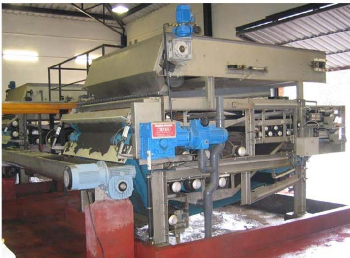
Pressure belt filters BS - BSPP - OS - OSC - MS are continuous cycle filters, which press the sludge by means of two belts which are entrained by a drive with adjustable speed. Each cloth comes with a spraying tube which washes the cloth in a continuous way.
