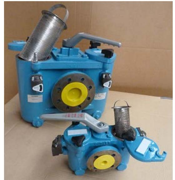
**BASKET FILTERS:** These can use one or two baskets and their use is mainly for retaining big particles.
