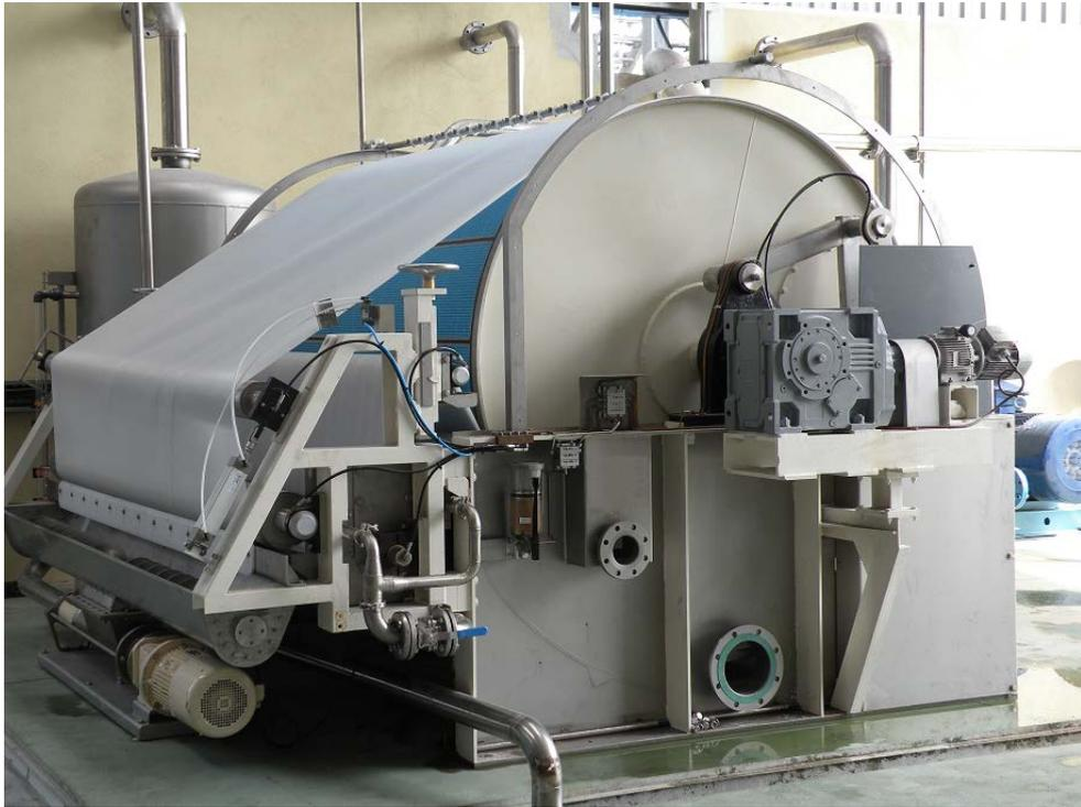
The drum filter is another type of continuous operation filter. The main difference in this case is that it allows different types of discharge systems according to the filtrated product.
