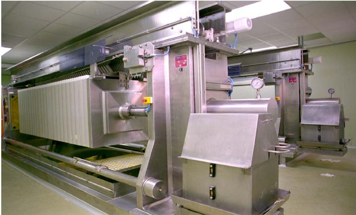
The cable overhead PSEH filter presses have been designed with a transport system which does not require any greasing. This makes them highly suitable for very corrosive environments such as acid industry, metal refineries and clean environments such as food industry, pharmaceuticals, oil refining, greases, agar and carrageenan, among others.
