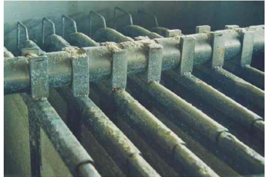
**Leaf filters** are suitable for low solid concentration products, high temperatures, easily oxidizable products, dangerous or polishing filtrations with precoat.
